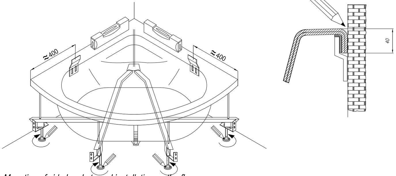
3. Mounting of side brackets and installation on the floor
